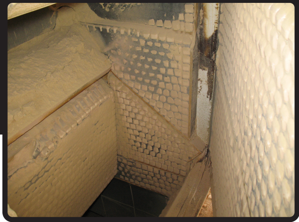
HardCube Liners in this engineered TripleGate Feeder handle the extreme conditions of impact and abrasion for years.
