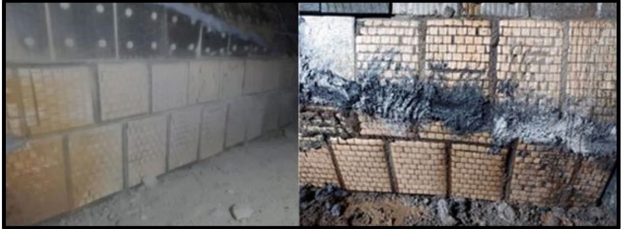
Left: Liners after two months; Right- Liners after 17 month and still in excellent condition.
