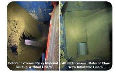
These systems are **cost-effective** when deployed in areas prone to severe buildup due to high moisture content in the material. They involve rubber liners that are inflated using plant air, regulated through a control box to maintain low pressure before passing through the liner system. Such an approach ensures prolonged, maintenance-free service periods, significantly boosting operational efficiency.
