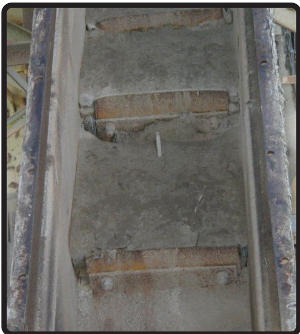
AR Steel Liner
