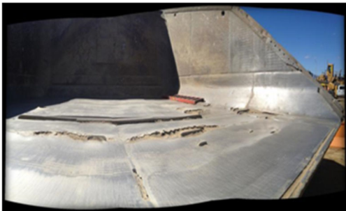
Common fractures and liner damage in truck boxes with steel liners.
