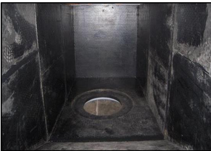
Launder Liners with Rubber-Ceramic held in place with internal magnets – no holes or hardware needed.
