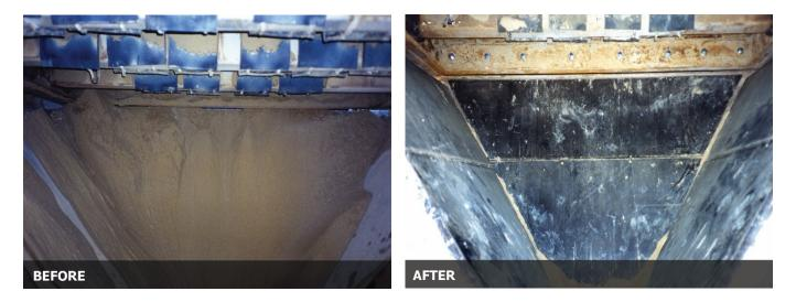
(Before) An example of a chute backed up by sticky material buildup. After Valley Rubber's liners were installed the chute was clear and functional.
