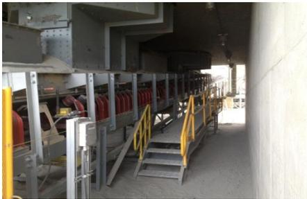
**Solution:** Valley Rubber's solution included adding BeltSeal Clamps with DoubleLip DustSeal skirting and Impact Idlers that are spaced tighter together. Adjustable BeltStabilizer Brackets and Bars were installed between the troughing idlers. A BeltSeal-Kit and TailSeal-Kit were installed, and the three-man cleanup crew now only had to come once every two weeks.
