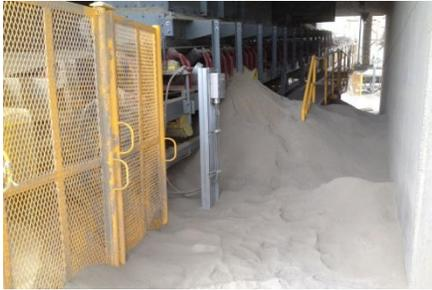
An operation's load zone was not properly supported which allowed the belt to porpoise between the impact idlers. Significant spillage, dust and maintenance resulted from this issue. The Load Zone was running 3000TPH with two Cone Crushers at 1,100hp each, crushing 14" minus material to ¾" minus. A three-man crew spent six hours twice a week cleaning up the spillage.
