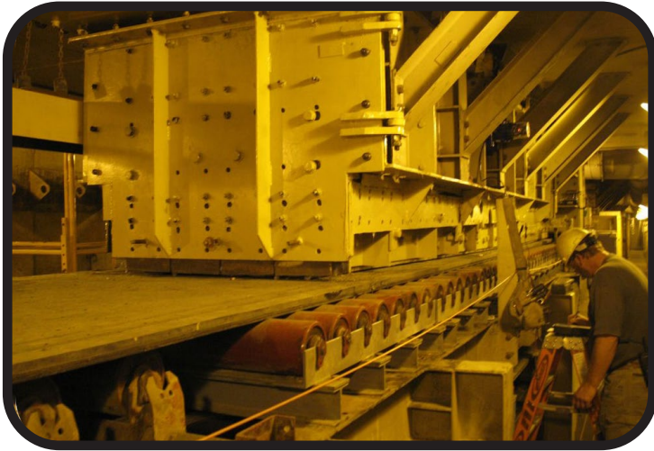
These feeders were fitted with an internal Loading Shoe and a Roller Table.
