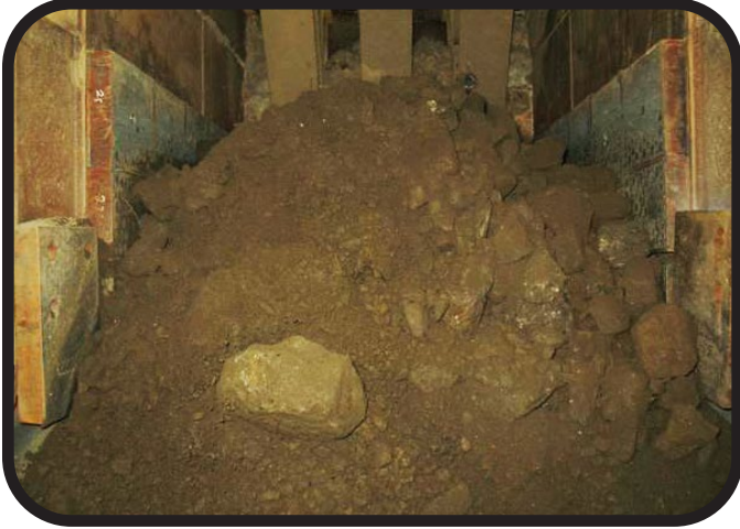
800 TPH of primary crushed ore.
