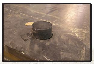
Rubber plugs are provided for each counterbored hole to protect the hardware. Use a little water on the plugs to make them slip in easier.
