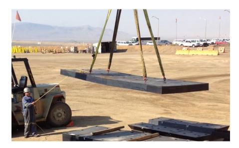
Lifting lugs (4), as shown below, are provided as part of the hardware package for every liner set and must be used for all lifts. The  $\emptyset 3/4$ "-NC x 2" long hex bolts required for bolting to the lift points are provided as part of the kit.
