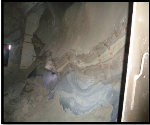
Photos above: Extreme plugging due to the failure of a competitor's inflation system.
