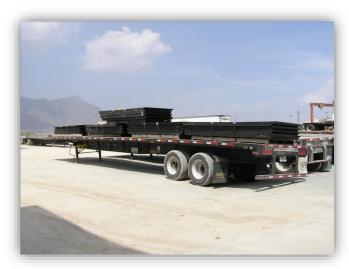
Each liner has threaded lugs to attach eye bolts for ease of lifting and positioning liners. Each system comes with an easy to follow liner map that directs the placement of each piece. The first liners to be installed are nearest the cab and typically have beveled edges where they meet the walls; once these are positioned with the help of a boom, the remaining liners should be placed next to the previous liner snugly.
