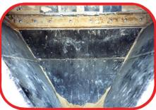
Cost Effective when installed in areas where there is severe buildup as a result of high moisture content in the material. These systems consist of rubber liners inflated by means of using plant air fed into a control box and reduced to low pressure prior to passing through the liner system. These systems provide extensive periods of maintenance free service in areas which were previously high upkeep and downtime.
