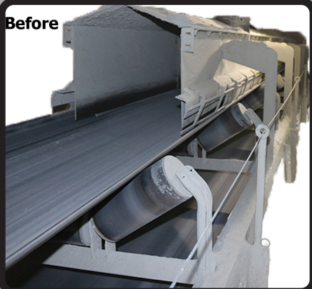
The original design allowed material and dust to escape between the belt and canoe.
