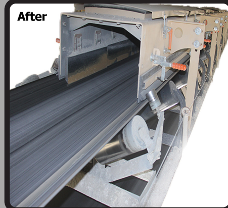
The new design includes all of Valley Rubber's BeltSeal-Kit components.
