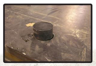
Rubber plugs are provided for each counterbored hole to protect the hardware. Use a little water on the plugs to make them slip in easier.
