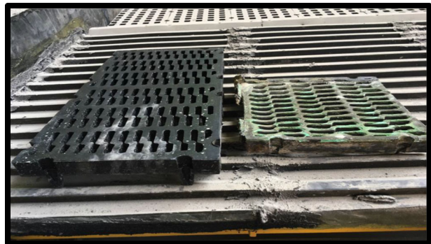
Photo Above (Left) Valley Rubber Screen (Right) Screen used prior to Valley Rubber.
