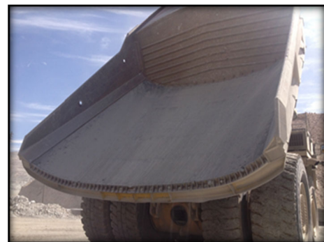
Komatsu 930 Haul Truck, five years of using rubber liners and still in service.
