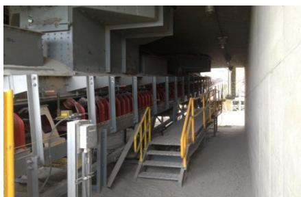
**Solution:** Valley Rubber's solution included adding BeltSeal Clamps with DoubleLip DustSeal skirting and Impact Idlers that are spaced tighter together. Adjustable BeltStabilizer Brackets and Bars were installed between the troughing idlers. A BeltSeal-Kit and TailSeal-Kit were installed, and the three-man cleanup crew now only had to come once every two weeks.
