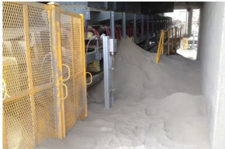
An operation's load zone was not properly supported which allowed the belt to porpoise between the impact idlers. Significant spillage, dust and maintenance resulted from this issue. The Load Zone was running 3000TPH with two Cone Crushers at 1,100hp each, crushing 14" minus material to  $\frac{3}{4}$ " minus. A three-man crew spent six hours twice a week cleaning up the spillage.
