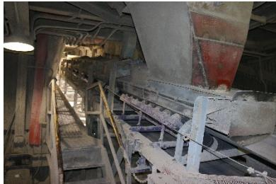
It is common to see either a piece of conveyor belt bolted to the rear of the canoe, or a slab of rubber bolted in the same fashion. Unable to be adjusted, these quick fixes are time consuming and rarely maintained, causing continued spillage and dust issues. The previous system pictured resulted in costly fines, excessive maintenance, loss of production and structural weight load concerns due to spillage.
