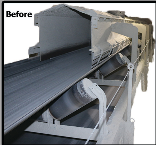
The original design allowed material and dust to escape between the belt and canoe.
