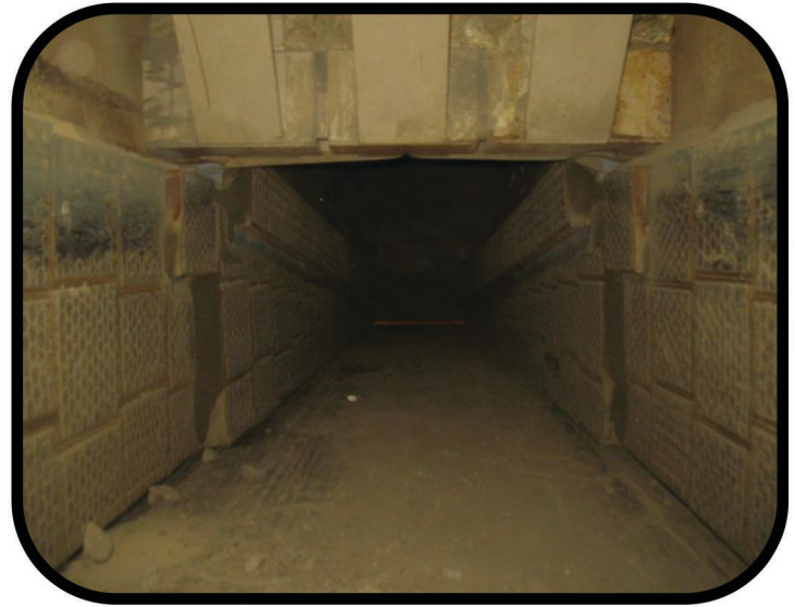
Internal Loading Shoe is fitted with ceramic liners on the Feeder Walls. Strike-off bar is overhead.
