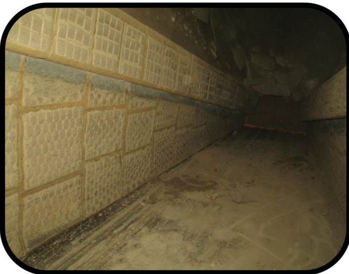
Looking toward the tail of the Loading Shoe. Top left is the engineered ceramic Deadbed Bar that protects the tapered floor of the Shoe.
