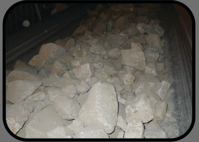
Approximately 1,600 TPH of SAG mill feed. The rocks are sharp, hard and angular.
