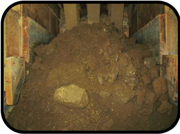
800 TPH of primary crushed ore.
