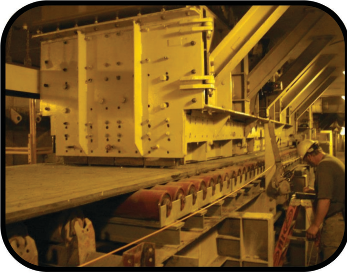
These feeders were fitted with an internal Loading Shoe and a Roller Table.
